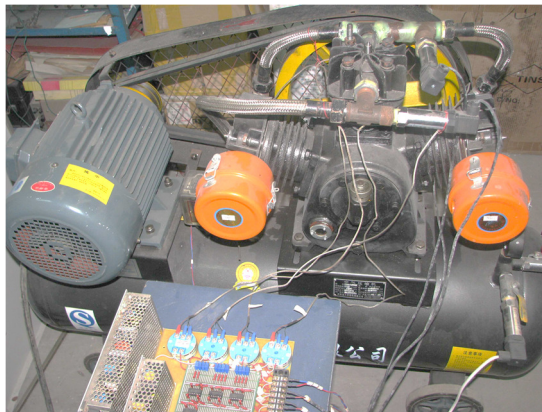
Fig. 2. Reciprocating compressor test platform
