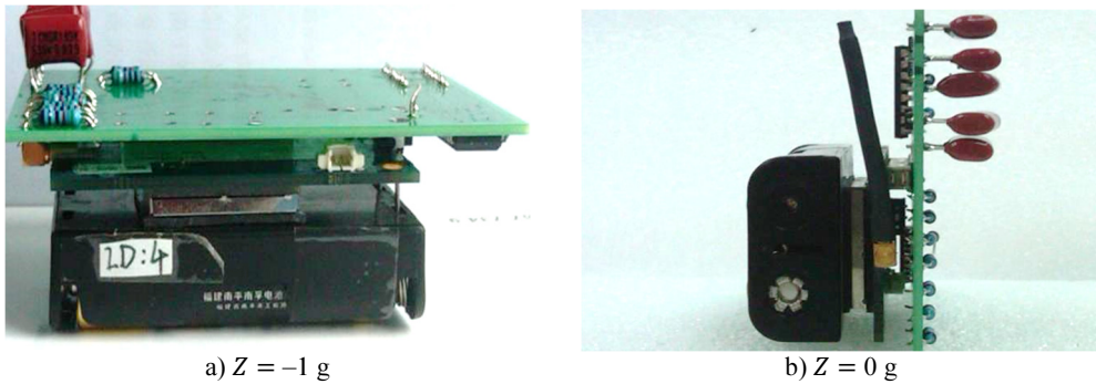
Fig. 7. Illustration of orientation for accelerometer calibration
