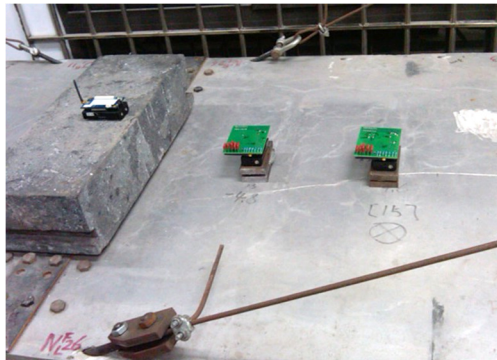
Fig. 13. Deployment of IRIS-Mote with the extension sensor board
