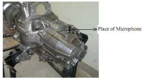
Fig. 3. The positioning of the acoustic sensor
