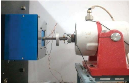
Fig. 9. The electromagnetic vibration exciter for the experiment
