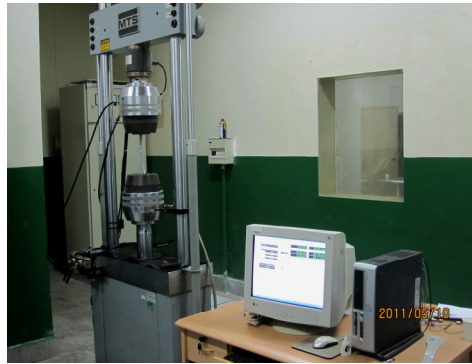
Fig. 3. Fatigue test system
