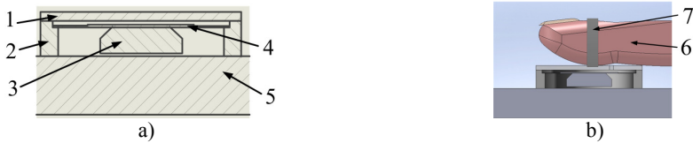
Fig. 8. Piezoelectric disc actuator with mass: a) cross section, b) 3D model. 1 – cover, 2 – plastic ring, 3 – additional element, 4 – piezoelectric disc actuator, 5 – PC screen, 6 – finger, 7 – rubber ring
