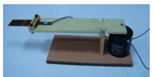
Fig. 2. Experimental platform of vehicle-vibration harvesting output power for the NQ45N smart material
