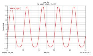
Fig. 8. Variation of toe in angle with sinusoidal bump input
