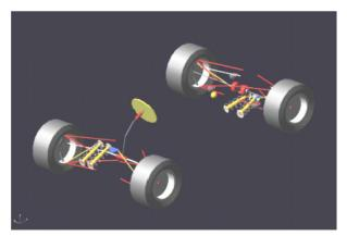
Fig. 12. Modeling of suspension system with steering in ADAMS
