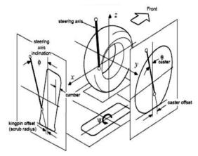
Fig. 1. Geometric parameters of tire
