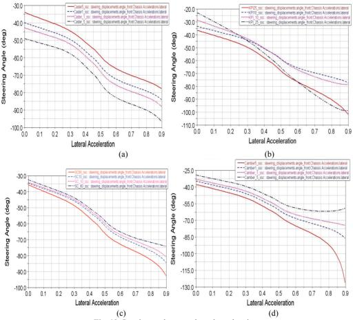
**Fig. 10.** Steering angle versus lateral acceleration: a) different caster angles; b) different kingpin slopes; c) different scrubs; d) different camber angles
