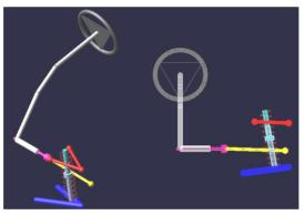
Fig. 5. The integrated DW suspension with steering system modeling
