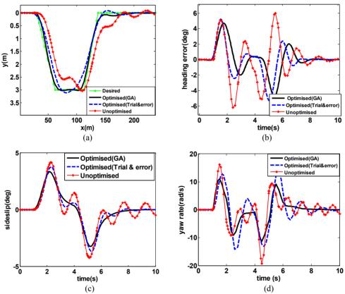
**Fig. 13.** a) Double lane-change maneuver path; b) vehicle heading error during double lane-change; c) vehicle side-slip angle during double lane-change; d) yaw rate variations during double lane-change
