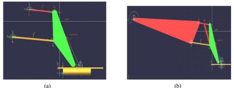
Fig. 6. Equivalent mechanisms of DW suspension system in ADAMS: a) bump input; b) roll input
