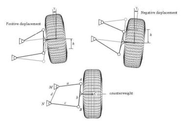
Fig. 2. Different types of camber angle resulted from wheel oscillations
