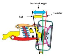
Fig. 4. DW suspension camber and steering angle [18]
