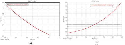
Fig. 7. Camber angle variation due to: a) bump; b) vehicle roll
