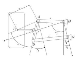
Fig. 3. Double wishbone suspension system and its geometric parameters [17]
