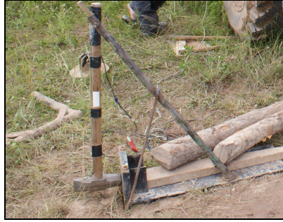
Fig. 3. Plate used for excitation of shear waves
