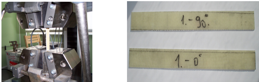
Fig. 6. Composite material sample during the test. Photo of test samples
