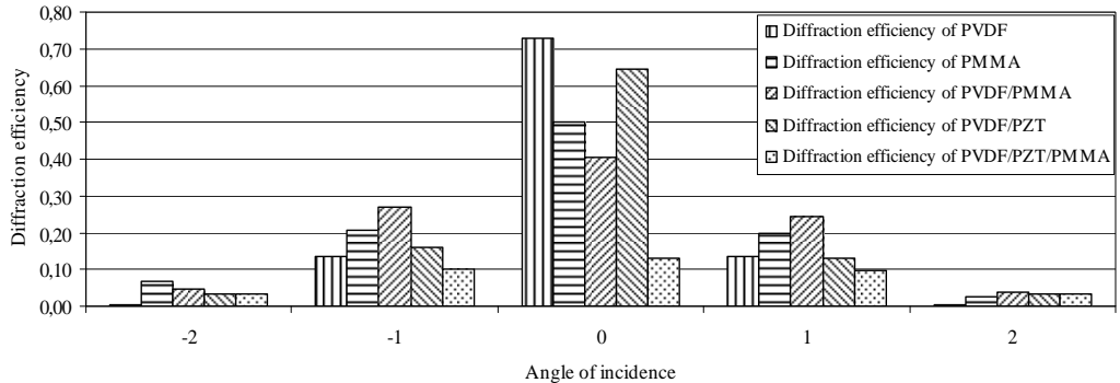
Fig. 4. Diffraction efficiencies of gratings imprinted on investigated thin film layers
