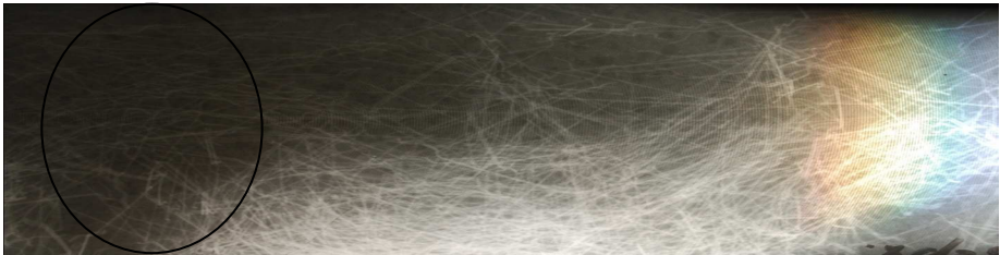
Fig. 6. X-ray image of fiber-concrete prism view from the side (fracture)
