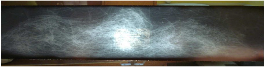
Fig. 5. X-ray image of fiber-concrete prism view from the side (location of fiber)
