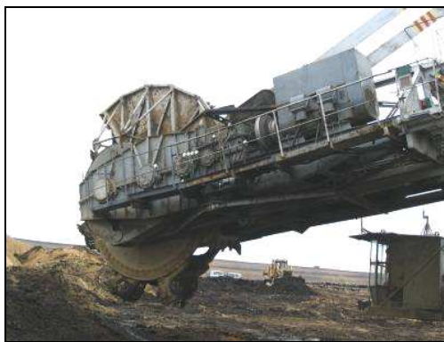
Fig. 1. Bucket wheel drive at the excavator SRs470.17/1.5 (400 kW)
