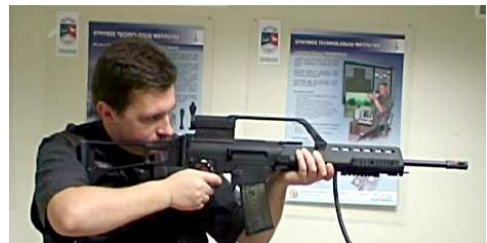
Fig. 5. Training weapon G36 with one way pneumatic drive
