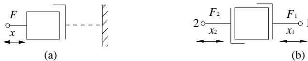
Fig. 4 Graphical symbols of two mass devices. (a) represents the mass element and (b) is the mass-like element, the two-terminal mass
