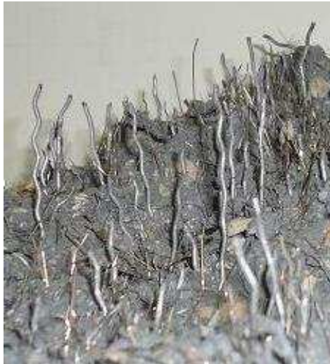
Fig. 3. a) Crack surface with pulled out steel fibers
