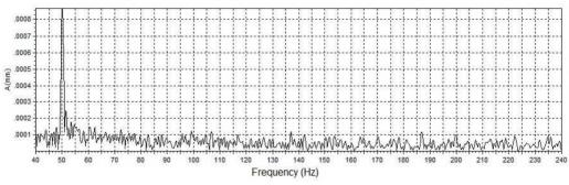
Fig. 6. Fourier spectrum of displacement oscillations with 50 Hz pressing force
