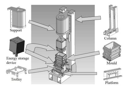
Fig. 1. Two-sided vibro-impact press
