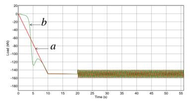
Fig. 4. The example of required (a) and implemented (b) pressing force function
