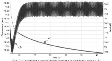
Fig. 7. Registered plunger displacement (a) and force graphs (b)
