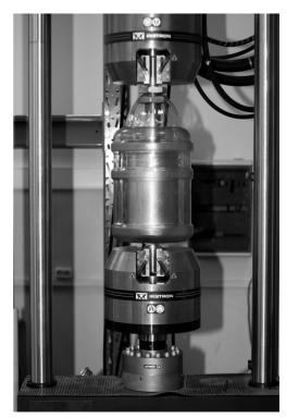
Fig. 3. Mold and plunger fixed in testing machine grips
