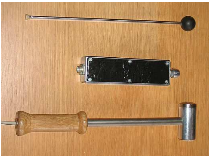
Fig. 7. Varieties of used impact type exciters
