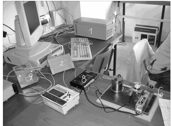
Fig. 1. Cantilever beam with sensor and controller
