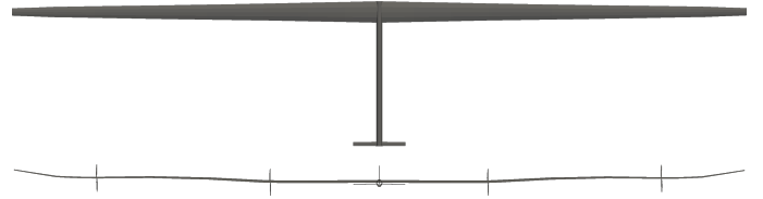
Figure 8: Top and rear view of the optimized single boom solar aircraft design during design operation.
