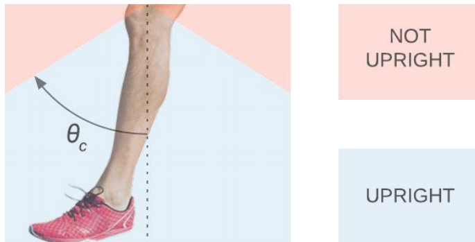
Fig. 2. The angle of each lower leg is compared to the critical angle ( \theta_c ) to determine uprightness.
