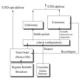
Figure 1: Algorithm Architecture.
