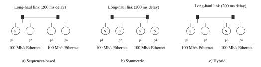
Figure 6: Protocol configurations.
