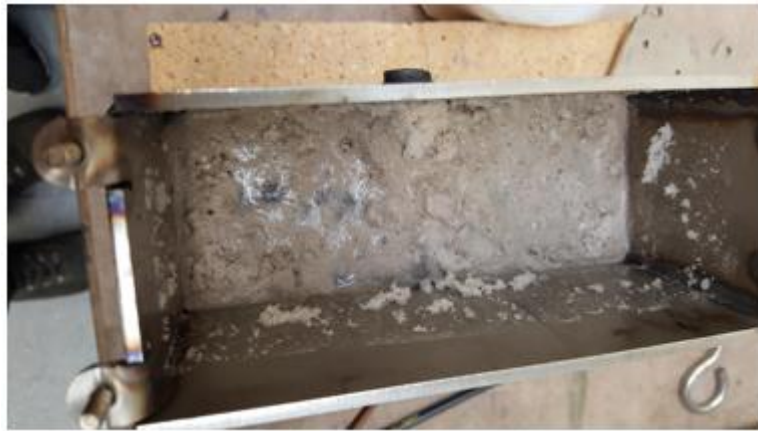
Figure 3-16: Filling a conventional stainless steel container with pure solar salt.
