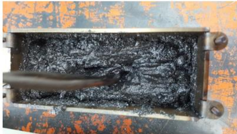
Figure 3-17: Filling the stainless steel finned container with solar salt.
