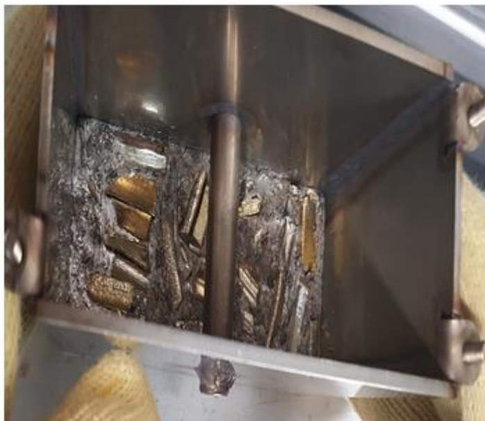
Figure 3-19: Filling the stainless steel container with Bi and Sn to form the PCM.
