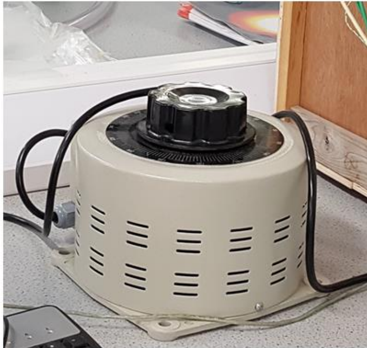
Figure 3-30: The electrical power input regulator.
