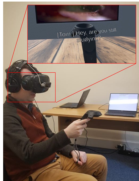
Figure 1: A TV viewer in VR wearing a head-mounted display, and headphones for the audio. The figure shows one out of five conditions ( controller messages ). Users receive text-messages directly on a HTC VIVE controller. The controller grabs users attention with a 1 s haptic feedback.
