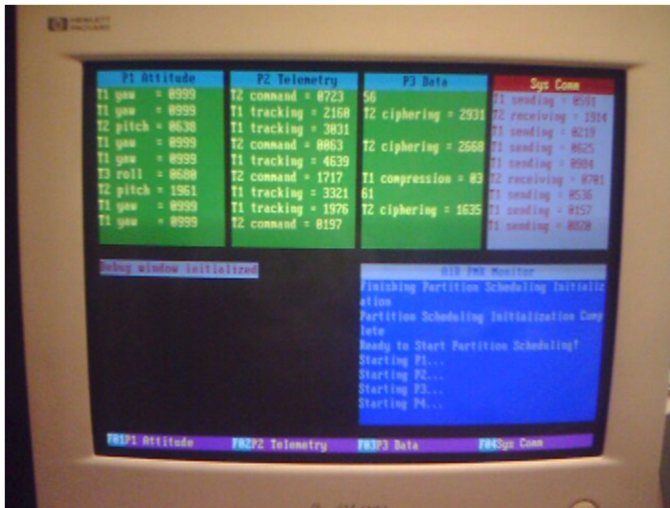
Figure 23 – The VITRAL visualization environment as used in the AIR proof of concept prototypes
