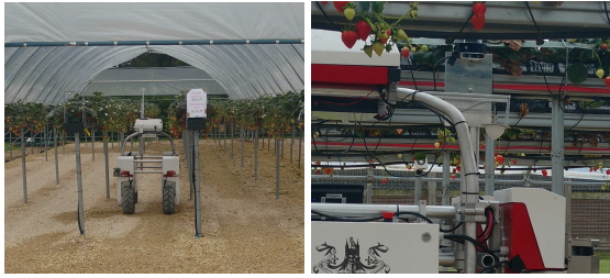
Figure 1: The strawberry farm, with a robot roaming in the tabletop rows collecting data (left). The sensor set-up used for data collection (right).
