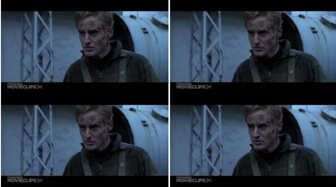
(b) Samples of "Video_1" compressed by our proposed technique HD-Coding (i.e. each image compressed independently, total compressed video size= 1.99 Mbytes), Average RMSE = 7.4. (See Table 2)
