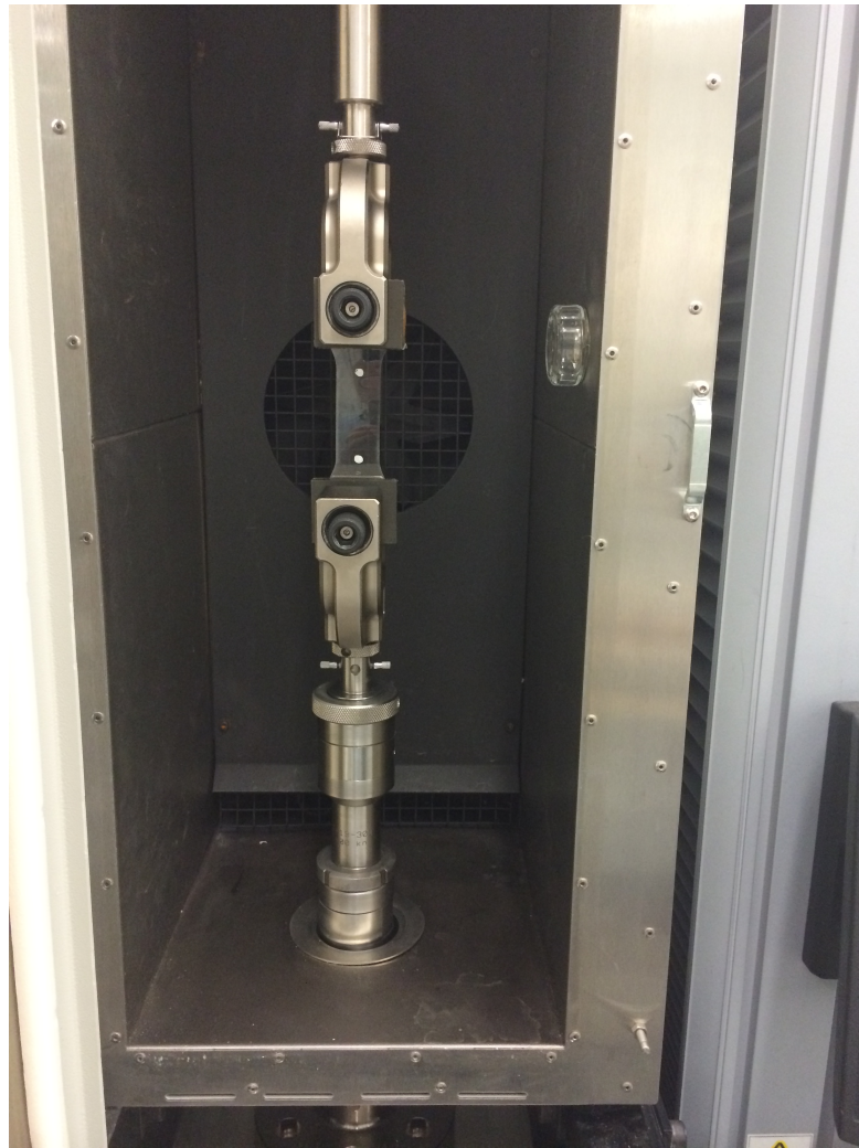
FIGURE 3.18: Pictures of a PMMA sample which was clamped in the environmental chamber. The two white dots setted the length of gauge length and were recorded by the video extensometer to calculate the axial strain (engineering strain).
