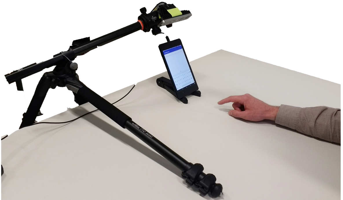
Figure 3.3: Layout of the prototype in-situ. A mounted camera overlooked the interaction area created in front of the mobile device.
