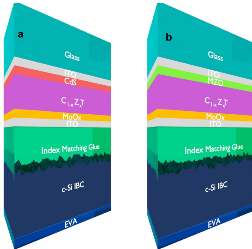
Figure 2. Schematic of C_{1-x}Z_xT/c\text{-Si} interdigitated back contact (IBC) tandem cells with top cell electron transport layers (ETLs) of CdS (a) and Mg_{0.23}Zn_{0.77}O (b).
