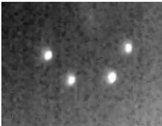
Fig. 4. Thermal picture of 4 impacts with .22LR, the rise in temperature is ca. 10 °C which can easily be detected.
