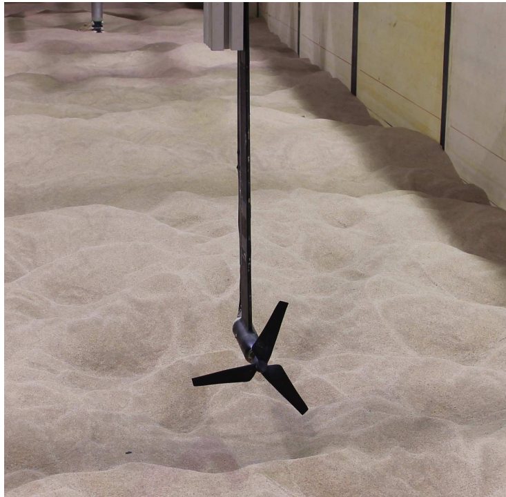
Figure 2: Hydrokinetic turbine with The three blades measuring 0.2 m diameter used during the experiments of Particle Image Velocimetry and mobile bed.
