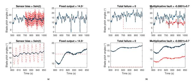
**FIGURE 8** Three pitch measurements from faulty (pitch 1) and fault-free (pitch 1 & 2) pitch sensors with the CPC pitch controller under wind condition WC1. (a) shows pitch measurements for the cases of either bias or fixed output sensor faults, (b) shows pitch measurements for the case of a total sensor fault (sensor failure) or for a multiplicative sensor fault.
