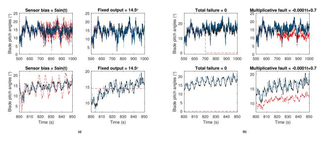
**FIGURE 9** Three pitch measurements from faulty (pitch 1) and fault-free (pitch 1 & 2) pitch sensors with the LQR-based IPC pitch controller under wind condition WC1. (a) shows pitch measurements for the cases of either bias or fixed output sensor faults, (b) shows pitch measurements for the case of a total sensor fault (sensor failure) or for a multiplicative sensor fault.
