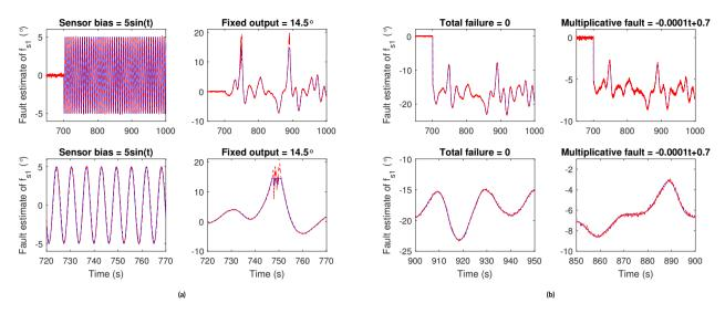
**FIGURE 10** Fault estimation results with the CPC pitch controller under wind condition WC1. (a) shows the estimation of fault  $f_{s1}$  for the cases of either bias or fixed output sensor faults, (b) shows the estimation of fault  $f_{s1}$  for the case of a total sensor fault (sensor failure) or for a multiplicative sensor fault.
