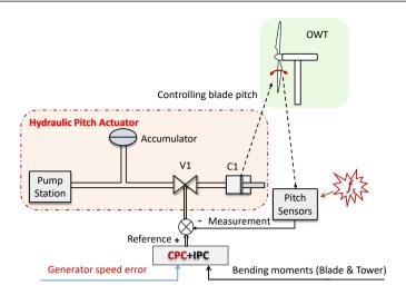
FIGURE 2 Wind turbine hydraulic pitch system
