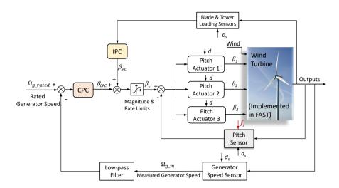
FIGURE 3 Considered pitch system structure with sensor faults
