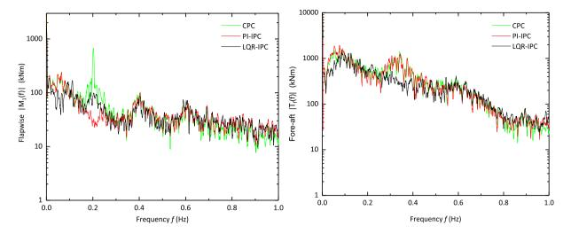
FIGURE 7 Frequency spectrum comparison of M<sub>1</sub> and T<sub>f</sub> with three different pitch controllers under wind condition WC1
