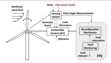
FIGURE 1 Fault-tolerant individual pitch control "co-design" scheme
