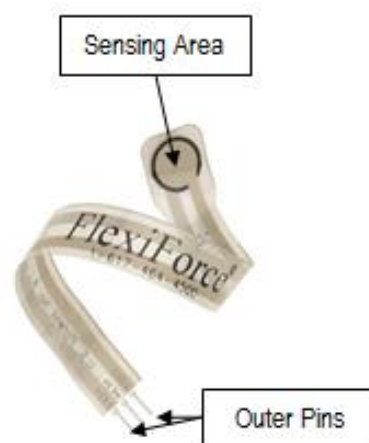
Figure 21 – FlexiForce force sensor is composed of small printed electrical circuits, which can be used for force measurements [42].
