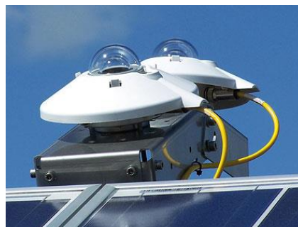
Fig. 1.18- Pyranometers on the tilted and horizontal planes
