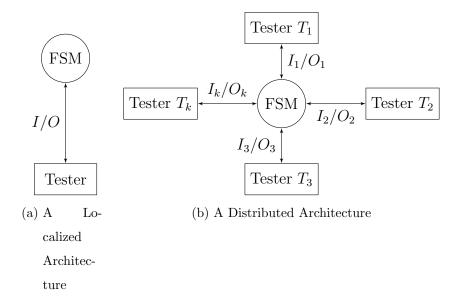
Figure 1.1.: Localized and Distributed Architectures
