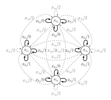
Figure 4.9.: The FSM  $M_D$  corresponding to the decision table given in Table 4.2
