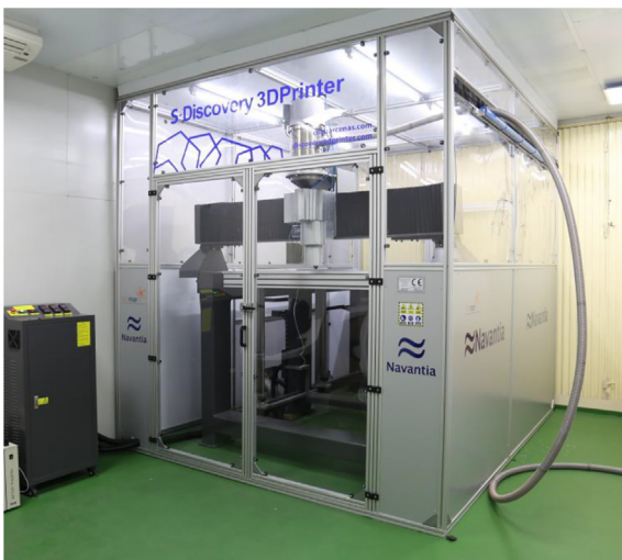
Fig. 3. S-Discovery LFAM device property of Navantia S.A., S.M.E. (placed at Bay of Cadiz Shipyard, Puerto Real, Cádiz, Spain). Adapted from [12].
