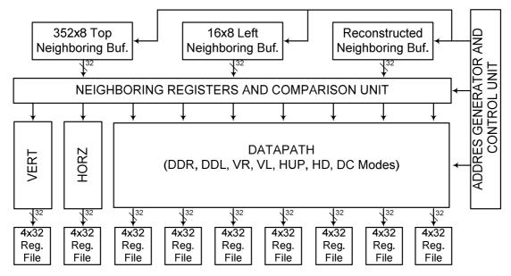
Figure 3.2 Top-Level Block Diagram of 4x4 Intra Prediction Hardware Architecture
