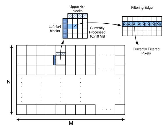
Figure 4.2 Illustration of H.264 DBF Algorithm
