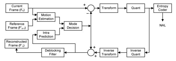
Figure 1.1 H.264 Encoder Block Diagram
