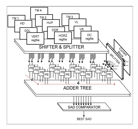
Figure 6.6 SAD Calculation PE Array and Adder Tree
