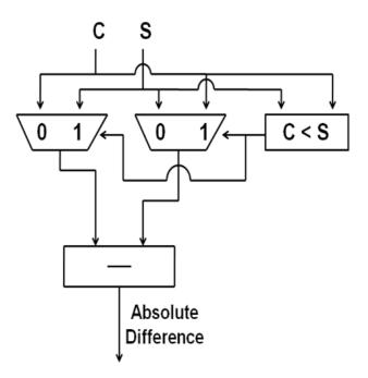
Figure 6.5 PE Architecture
