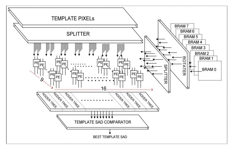
Figure 6.4 Template Search PE Array and 16 Adder Tree
