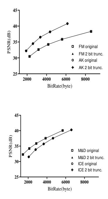
Figure 4.4 Rate Distortion Curves of the Original H.264 DBF Algorithm and H.264 DBF Algorithm with Proposed PSCR Technique
