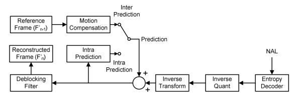
Figure 1.2 H.264 Decoder Block Diagram
