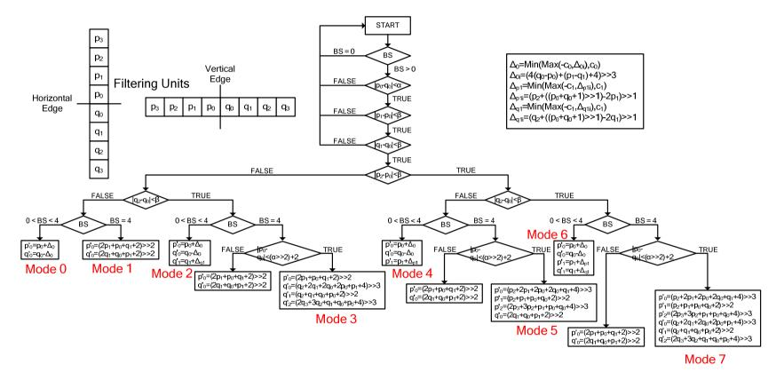
Figure 4.3 H.264 Deblocking Filter Algorithm
