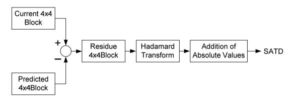
Figure 5.2 SATD Calculation for Each 4x4 Block
