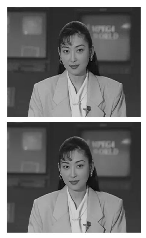
Figure 4.9 Unfiltered video frame shown above and the same frame filtered by H.264 Deblocking Filter algorithm shown below
