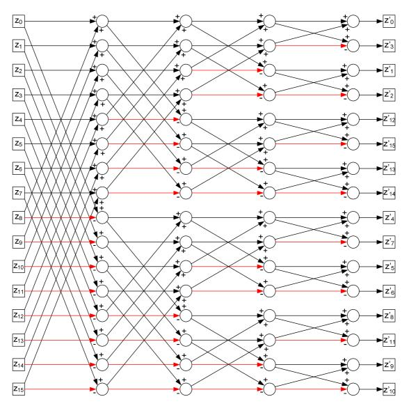
Figure 5.4 Fast HT Algorithm for a 4x4 Block
