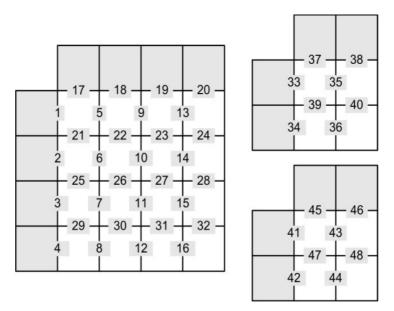
Figure 4.1 Edge Filtering Order Specified in H.264 Standard
