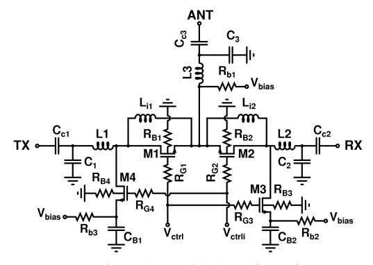
Figure 15: Circuit schematic of the designed SPDT T/R switch.
