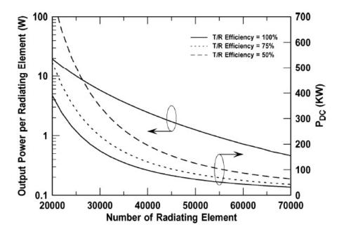
Figure 8: Output power per radiating element and total DC power required for all of the T/R modules versus number of elements for a fixed power-aperture-gain product [24].
