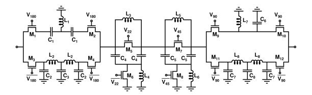
Figure 60: Layout of the X-Band T/R Module in IHP 0.25- $\mu$ m SiGe BiCMOS process.
