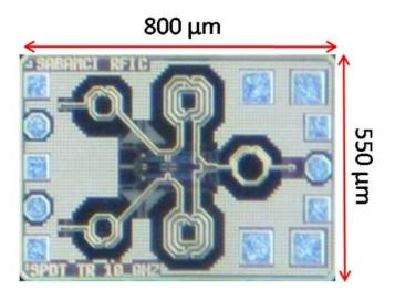
Figure 23: Die photo of the T/R switch. The chip area including pads is  $0.44 mm_2$ .
