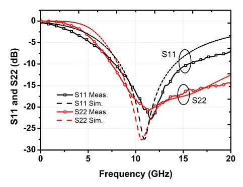
Figure 44: Measured  $S_{11}$  and  $S_{22}$  of the LNA (input and output matching).
