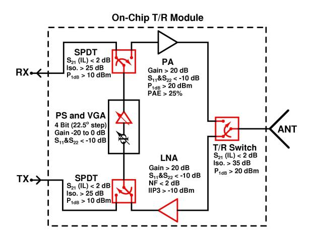
Figure 10: SiGe X-Band T/R module system block diagram. The highlighted blocks are the main focus of this thesis.
