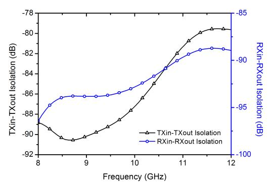
Figure 72: Simulated isolation of the transmit and receive modes.
