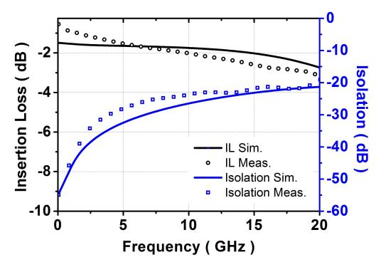
Figure 30: Measured insertion loss and isolation of the SPDT switch.
