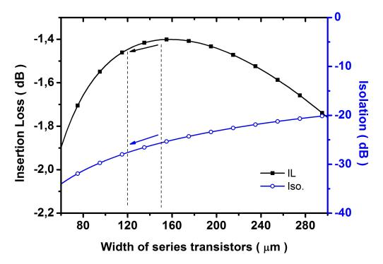
Figure 28: Simulated series transistor width versus insertion loss and isolation.
