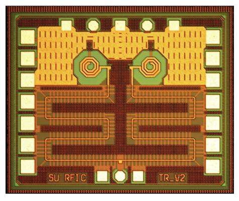
Figure 37: Die photo of the DC-20 GHz SPDT switch. The active chip area is  $0.48 \times 0.36 \ mm^2$ .
