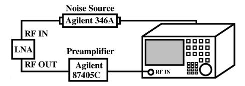
Figure 47: Measurement setup for noise figure.
