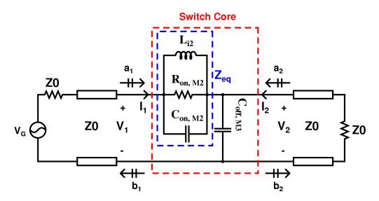
Figure 18: Circuit configuration to derive S21 of the ON transistor.
