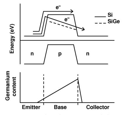
**Figure 9:** Ge concentration (bottom) and band structure (top) of a SiGe HBT. The Ge provides a lower barrier to injection from emitter to base as well as an accelerating field through the base.
