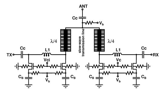
Figure 34: Schematic of the designed T/R switch using slow-wave transmission lines.
