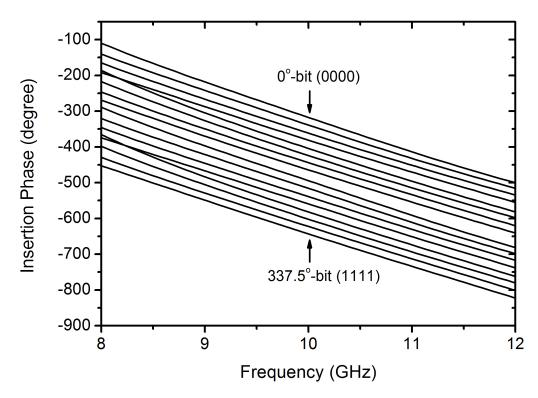
Figure 66: Simulated 4-bit phase response of the T/R module in the receive mode.
