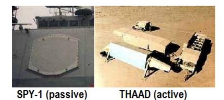
Figure 5: Photograph of a passive and active phased array radar
