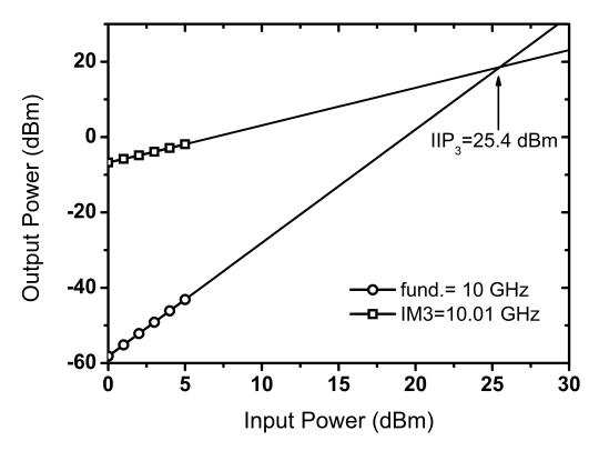
Figure 58: Input-referred third-order intercept point (IIP3) in bypass mode.
