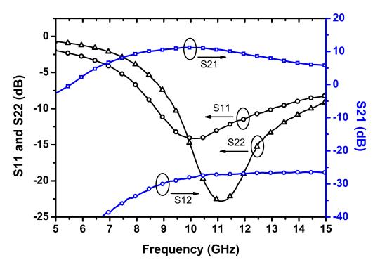
Figure 53: Measured S-parameters of the switched LNA in gain mode.
