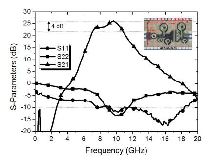
Figure 12: Measured small-signal gain and return loss of the two-stage power amplifier.
