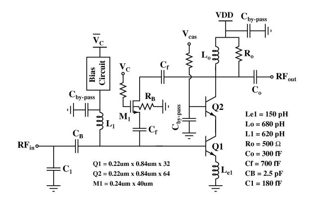
Figure 50: Circuit schematic of the switched gain LNA.
