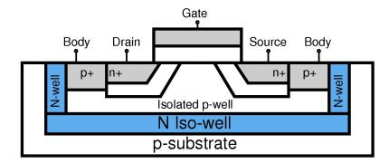
Figure 21: Cross-sectional view of a typical isolated NMOS transistor.
