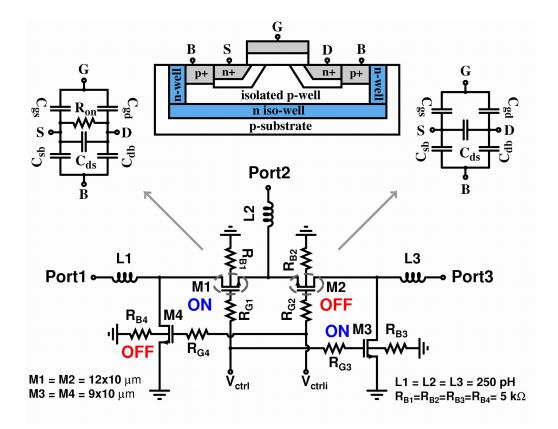
Figure 27: Circuit schematic of the designed SPDT switch and cross-sectional view of a typical isolated NMOS transistor.
