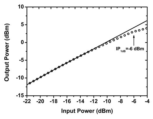
Figure 55: Measured P1dB of the switched LNA in gain mode.
