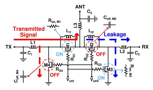
Figure 20: T/R switch in the transmit mode.
