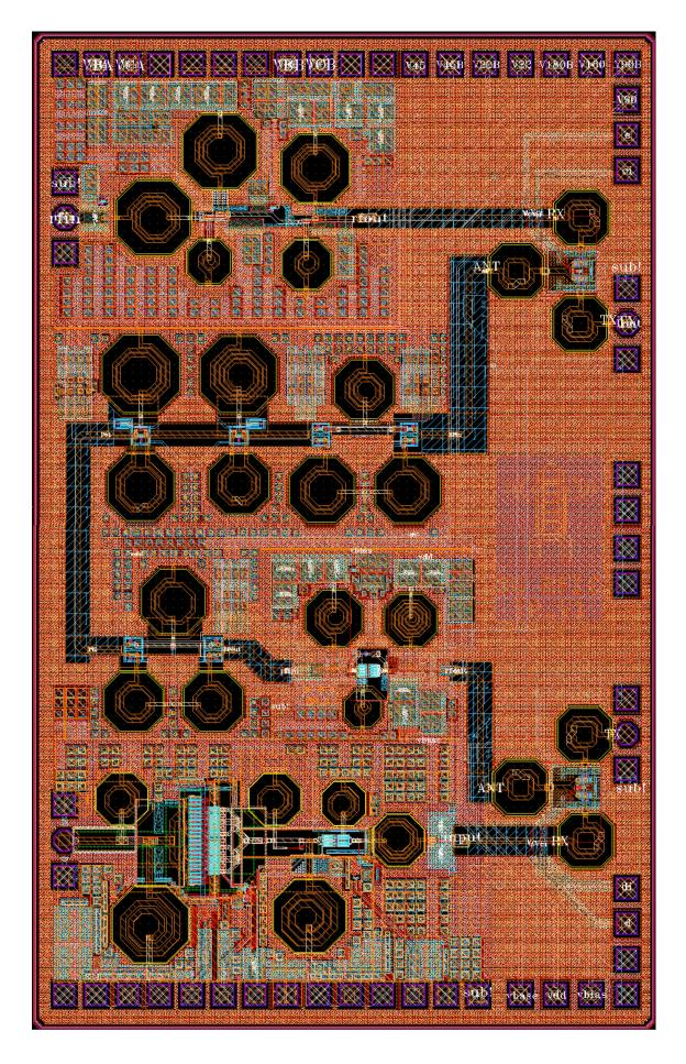
Figure 61: Layout of the X-Band T/R Module in IHP 0.25- $\mu$ m SiGe BiCMOS process. 72
