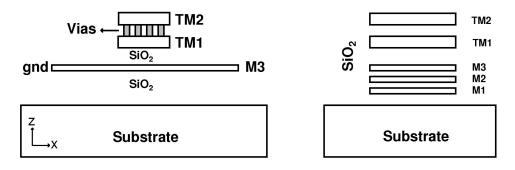
Figure 36: Simplified cross-section of the slow-wave transmission line and metal layers in the technology.
