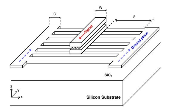
Figure 35: Structure of the slow-wave microstrip transmission line (S-MSL).
