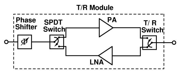
Figure 6: Simple block diagram of a solid state T/R Module
