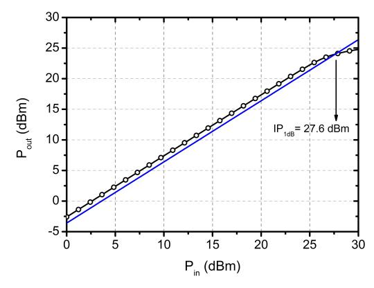
Figure 40: Measured 1 dB compression point  $(IP_{1dB})$  of the T/R switch at 10 GHz.
