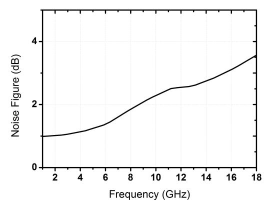
Figure 33: Measured noise figure of the SPDT switch.
