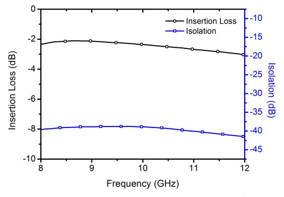
Figure 38: Measured insertion loss and isolation of the S-MSL based T/R switch.
