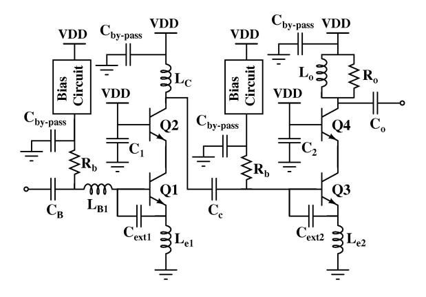
Figure 41: Schematic of the designed two-stage low noise amplifier.
