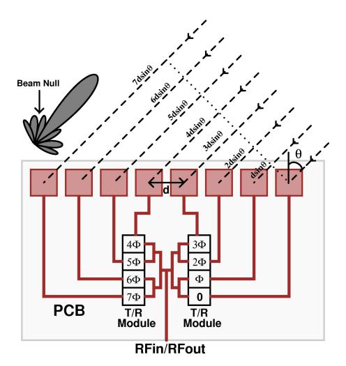
Figure 1: Phased array system with 8 antenna elements
