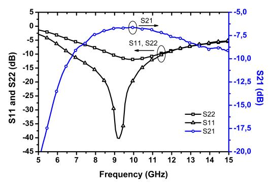
Figure 56: Measured S-parameters of the LNA in bypass mode.
