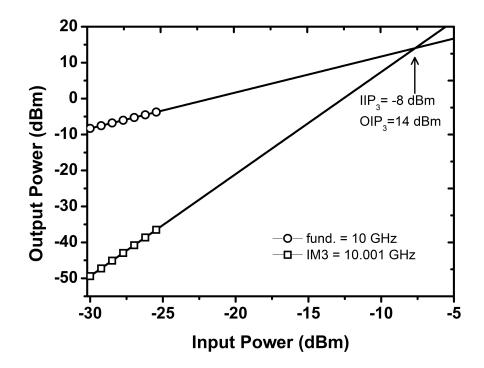
Figure 49: Measured input third-order intercept point.
