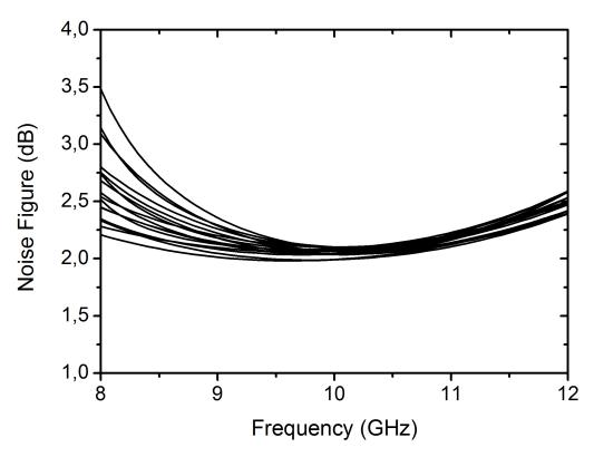
Figure 65: Simulated noise figure of the T/R module in the receive mode for all phase states.
