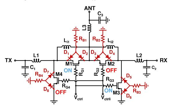
Figure 22: The switch core with body floating technique in TX mode.
