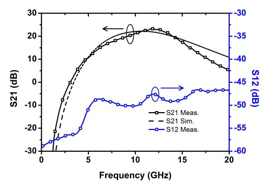
Figure 45: Measured  $S_{21}$  and  $S_{12}$  of the LNA (gain and isolation).
