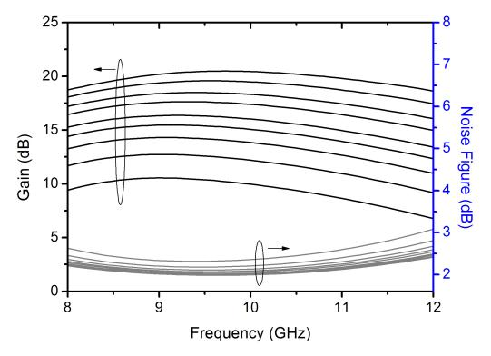
Figure 68: Simulated variation of the gain and noise figure of the T/R module in receive mode.
