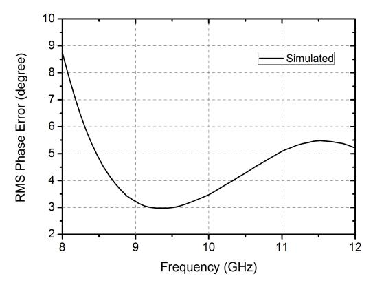
Figure 67: Simulated RMS phase error of the T/R module in the receive mode.
