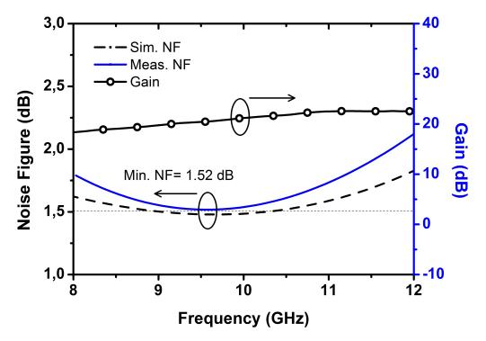
Figure 46: Measured noise figure and gain of the LNA across X-Band.
