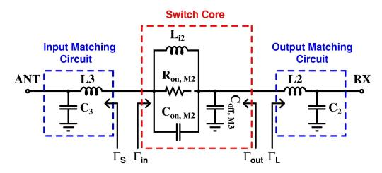
Figure 17: Transmit mode small-signal simplified model.
