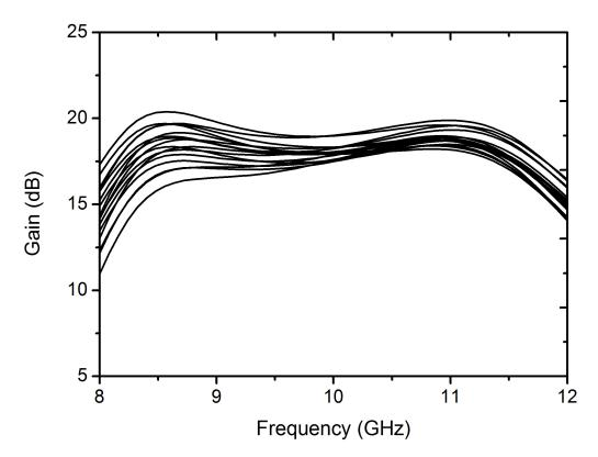
Figure 69: Simulated gain of the T/R module in the transmit mode for all phase states.
