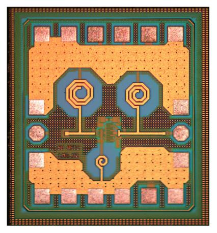
Figure 52: Die photo of the switched gain LNA. The active chip area, without pads, is  $0.52 \times 0.58 = 0.3 \ mm^2$ .
