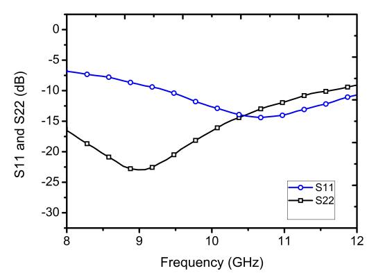
Figure 39: Measured return losses of the S-MSL based  $\mathrm{T/R}$  switch.
