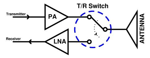
Figure 14: A simple block diagram of T/R module
