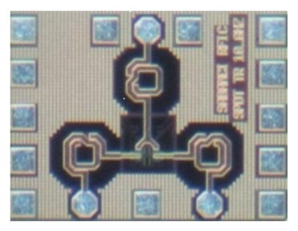
Figure 29: Die photo of the DC-20 GHz SPDT switch. The active chip area is  $0.48 \times 0.36 \ mm^2$ .
