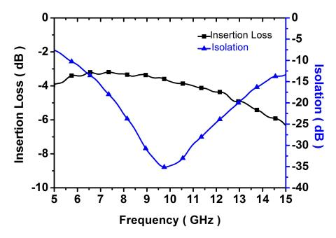
Figure 24: Measured insertion loss and isolation of the T/R switch.
