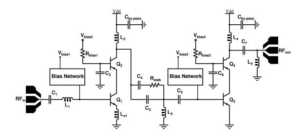
Figure 11: Schematic of the designed two-stage power amplifier.
