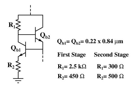
Figure 42: Schematic of the active bias circuit.
