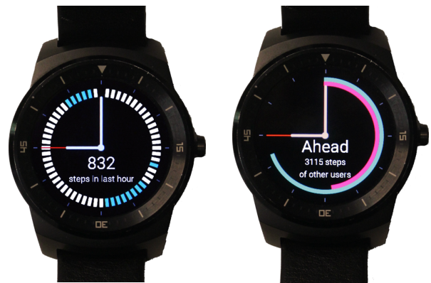
Figure 1 – TickTock (left) and Normly (right), two of the concepts developed as watchfaces. TickTock portrays periods in which one was physically active over the past hour. Normly compares one's goal completion to that of others having a similar walking goal.
