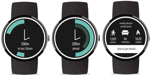
Figure 7. TickTock (left) visualizes physical activity of only the past half an hour, thus rendering feedback a scarce resource. Catchup (middle) enables competition with one’s past self through contrasting current goal completion (outer ring) to that attained at the same time yesterday (inner ring). Predicto (right) fosters surprise by predicting upcoming day’s walking distance from one’s sleep pattern, weekday physical activity patterns and recent walking tendencies.
