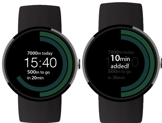
Figure 9. Mikro compares one’s progress to a micro-goal (outer ring) to the time remaining to complete a goal (inner ring). Mikro also allows users to make short adjustments to goals.
