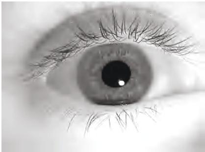
FIGURE 4: The iris image from Figure 1 after compression to 100 : 1.
