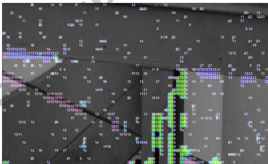
Figure Color map showing the vibration frequencies of the different parts of a pedestrian bridge. Notice the cable, deck and vertical beam vibrating at 10, 13 and 19 Hz respectively.
