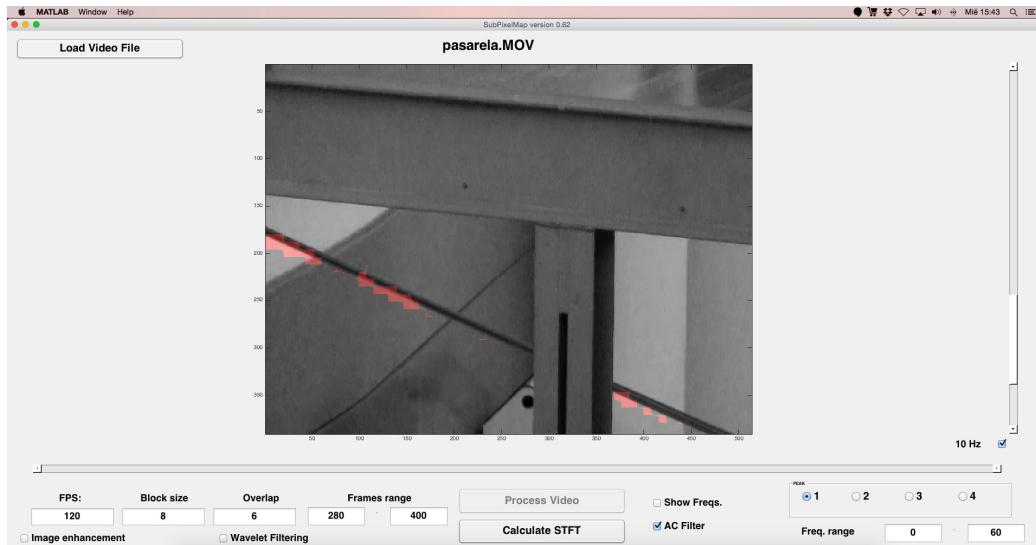
Figure 8 (video). Video sequence with the areas vibrating at a specific frequency highlighted in red. Notice the three main areas, cable, deck and vertical beam, vibrating at 10, 13 and 19 Hz, in accordance with the map in Figure 6. (See the video at https://goo.gl/D60saN )
