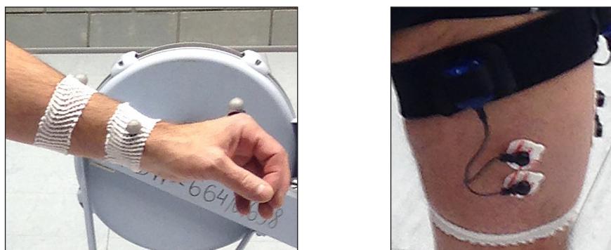
Fig. 3. Securing the glued markers with dressing mesh (a); EMG sensors with electrodes on the thigh (b)
