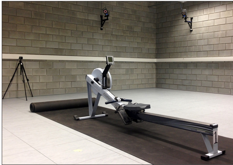
Fig. 1. The motion capture stand with an ergometer in the LARiEI room
