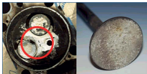
Figure 1: Deposits on the generator valves.
