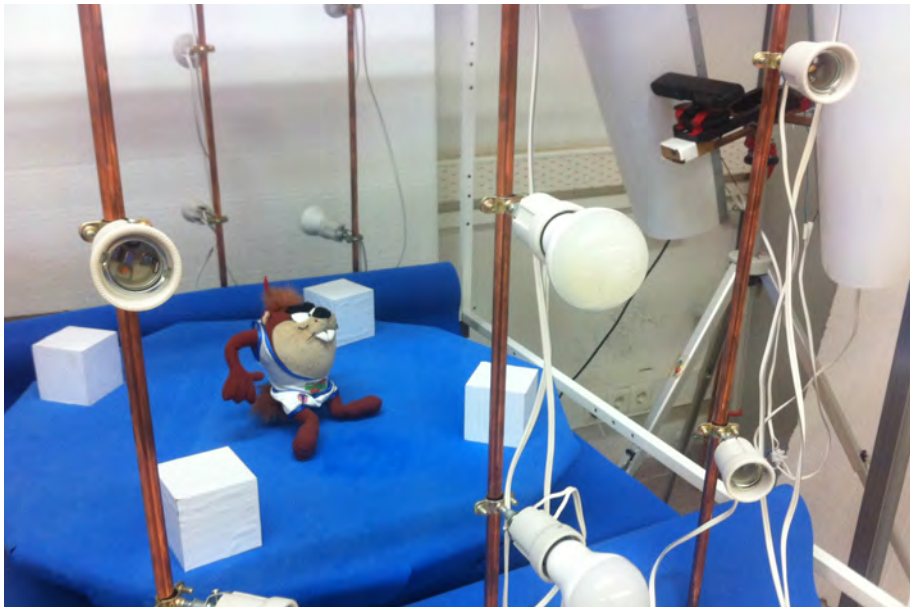
Figure 6: Real turntable set up for the real data experimentation. The markers are white cubes around the target object (a Taz toy).
