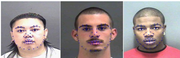
Fig. 5 Fiducial landmark detection results. Blue points represent the 68 landmark points
