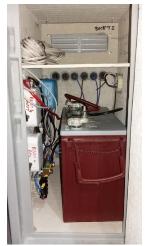
Figure 6: Battery, charger, monitor, relay, transmitters and inverter during bench tests (A: left) and installed in enclosure (B: right)
