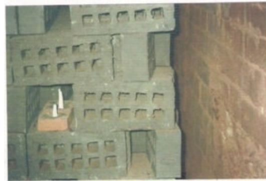
Plate 1 The position of the seger cone between stacked bricks inside the kiln
