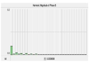
Figure 7. The current harmonics of phase B on 110 KV side.
