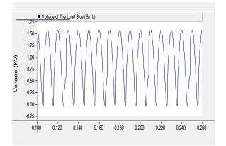
Fig. 3. Voltage waveform on 110 kV side of traction substation transformer.
