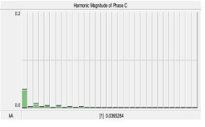
Fig. 11. The current harmonics of phase C on 110 KV side.
