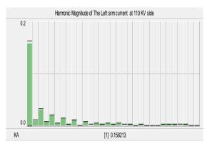
Fig. 5. Harmonics of the total current at 110 KV side.
