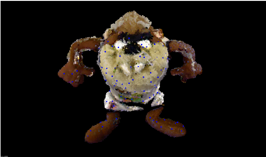
Figure 3.10: Keypoints extracted with ISS in blue (salientRadius = 6, nonMaxRadius = 4, minNeighbors = 5, threshold21 = 0.975, threshold32 = 0.975).
