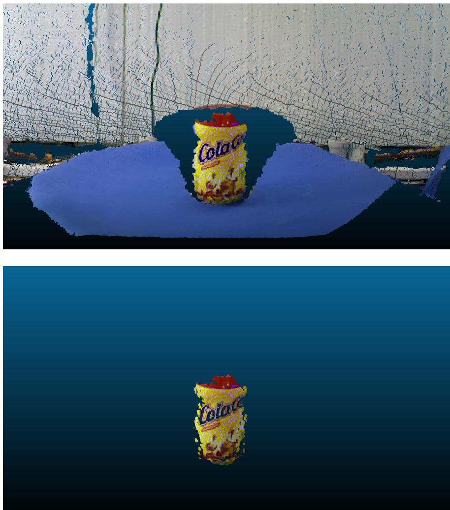
Figure A.4: Original point cloud of a partial view (top), segmented point cloud after preprocessing (bottom).
