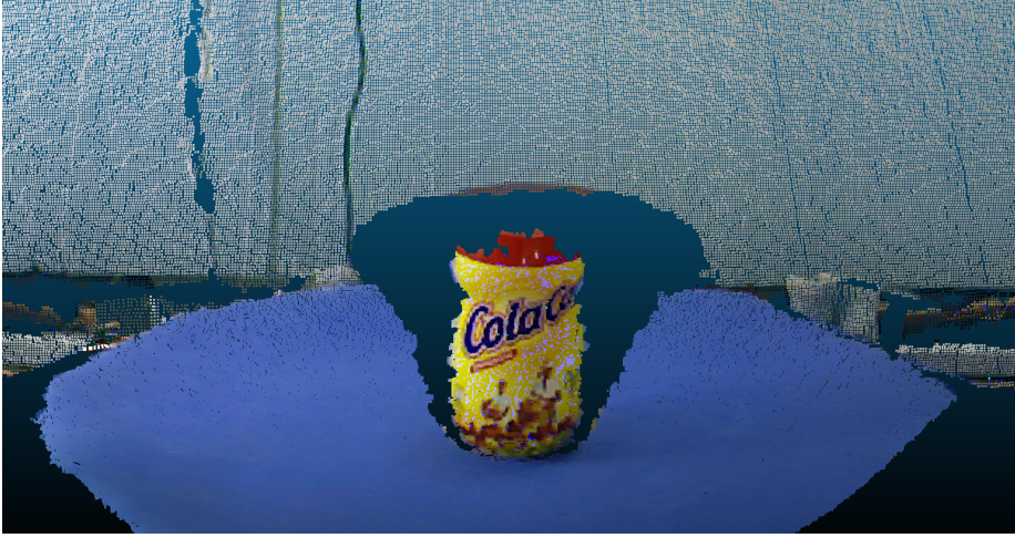
Figure A.1: Point cloud (XYZRGB) of a partial view of an object on the turntable captured using the aforementioned grabber with a PrimeSense Carmine device..
