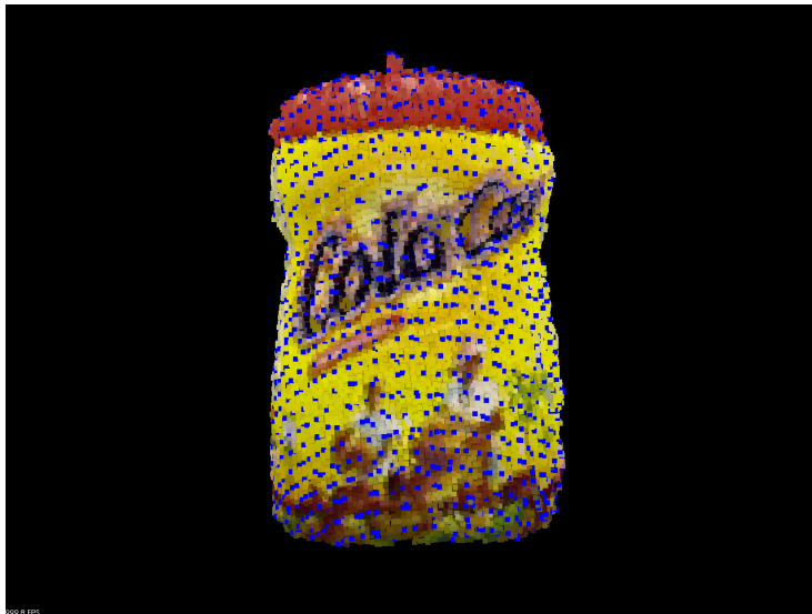
Figure 3.9: Keypoints extracted with uniform sampling in blue. Notice the low distinctiveness of the keypoints as they are detected everywhere.
