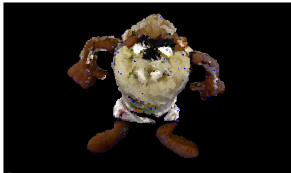
Figure 3.11: Keypoints extracted with SIFT in blue (minScale = 0.005, nrOctaves = 8, scalesPerOctave = 8, minimumContrast = 0.005).
